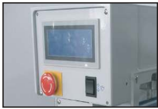
PLC control touch screen
