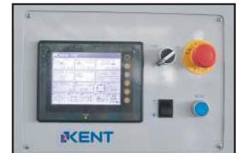
PLC control with touch screen interface
