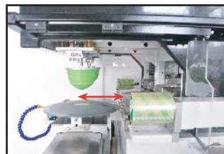
Plate in/out movement for maximum product clearance
