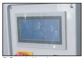
PLC control touch screen
